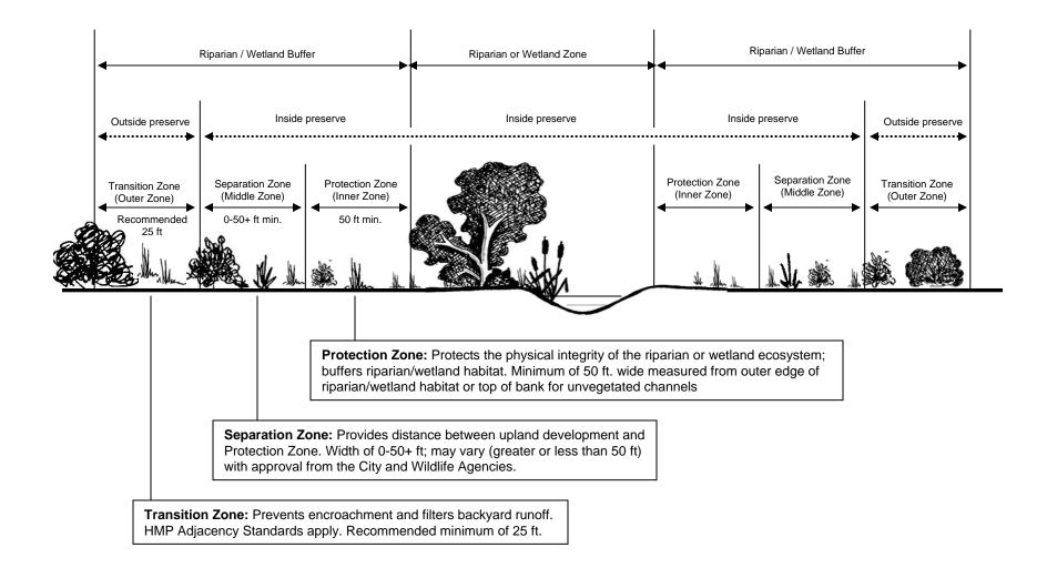
Figure 1. Protection, Separation, and Transition Zones
