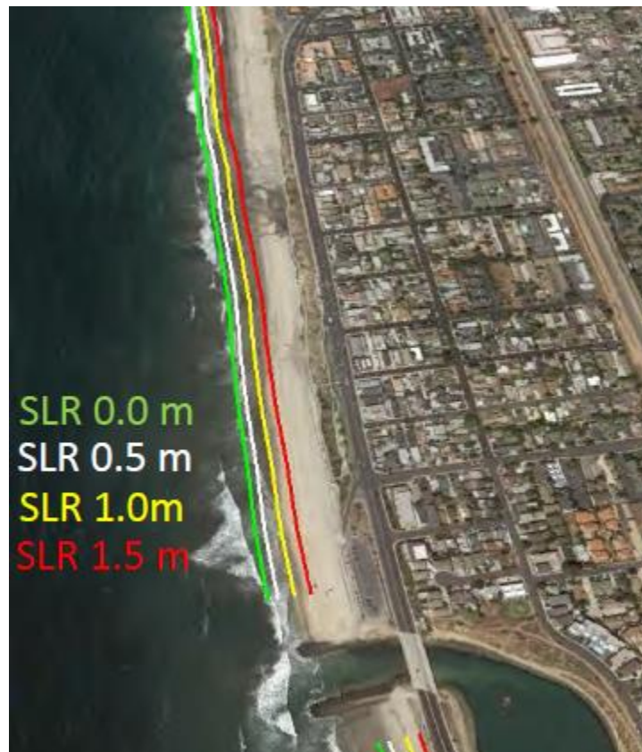
Figure 6: CoSMoS Shoreline Erosion Projections by 2100
